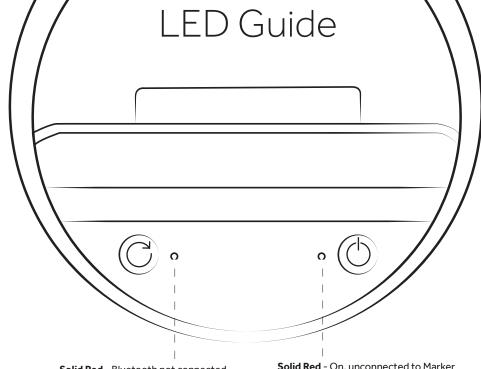
Solid Red - Bluetooth not connected Flashing Red - Bluetooth ready to pair Solid Green - Bluetooth connected
