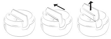
Finally, insert shim into grip holder and place in base.
